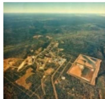
*Aerial view of the mining and refining site out of Kalgoorlie. Mine workings are on the left; refining plant in the center; tailings ponds and evaporation dams to the right. Note the greenness of the desert.*
